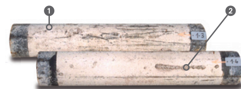
200 g/m 2 zinc + 80 μm bituminous paint coating
